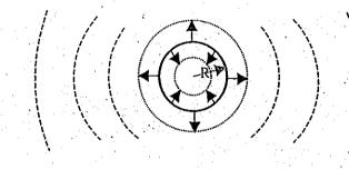
Oscillating bubble emitting high pressure pulses
