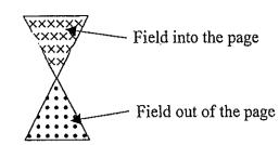
(ii) An electromagnetic force acts on an electron in the field making it move in the arc of a circle. The longer the electron stays in the field the greater its deflection, so the outer electrons (top and bottom) will be deflected through a greater angle than those near the centre because they pass through more area of the field during their motion.
