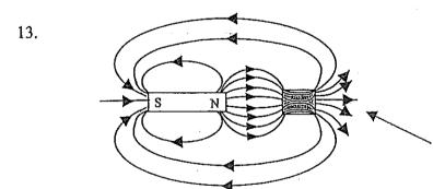
NB. The iron concentrates the magnetic lines of force and the field will return around the outside to the S-end of the magnet.
